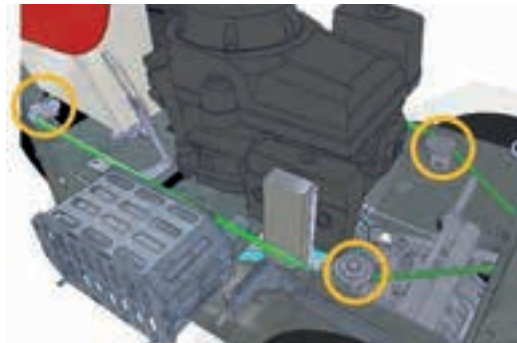
(Fig. 20 - Tensioning / loosening the roller chain)
