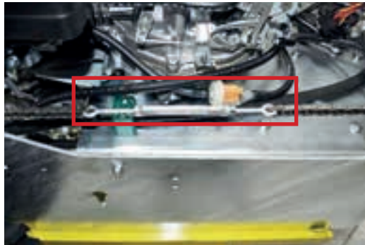
(Fig. 19 - Tensioning / loosening the roller chain)
