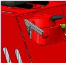
Fig. 19: Rotating speed regulation
